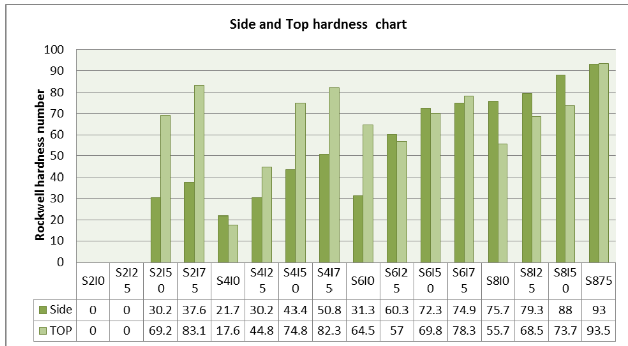
Figure 3.3: FDM specimen Side and Top hardness Chart
